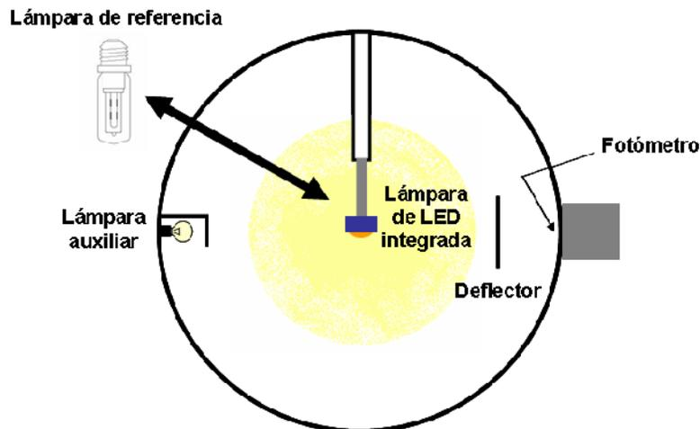
Figura H.2. Configuración de la esfera integradora  $2\pi$
