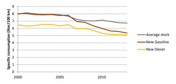
Figure 25 Specific energy consumption of average car stock, new gasoline cars and new diesel cars, 2000-2013 (liter/100 km)
